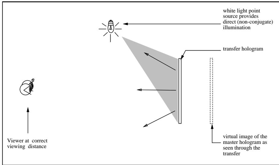
Figure 13: Viewing a direct-illuminated ULTRAGRAM.
