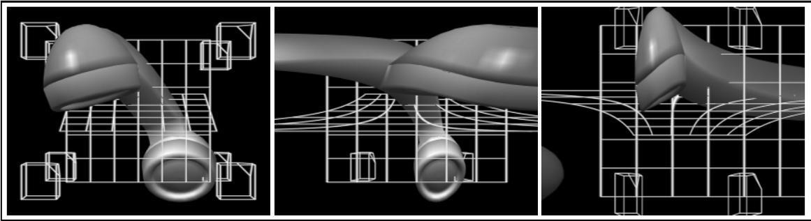
Figure 7: On the left is a single frame from a computer-generated three-dimensional test pattern. The center frame shows the effect of image predistortion where the holographic stereogram is to be illuminated in phase conjugate illumination. On the right is an image designed to expose a non-phase conjugate (direct) illuminated stereogram.
