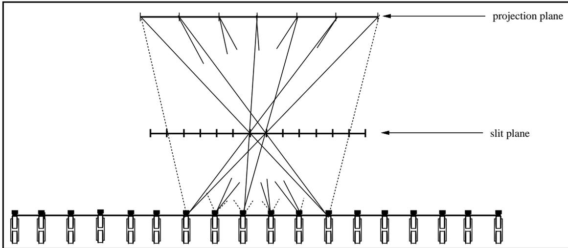
Figure 9: In perspective slicing, the projection screen image for each slit is formed by collecting the pieces of each camera view that pass through that slit.
