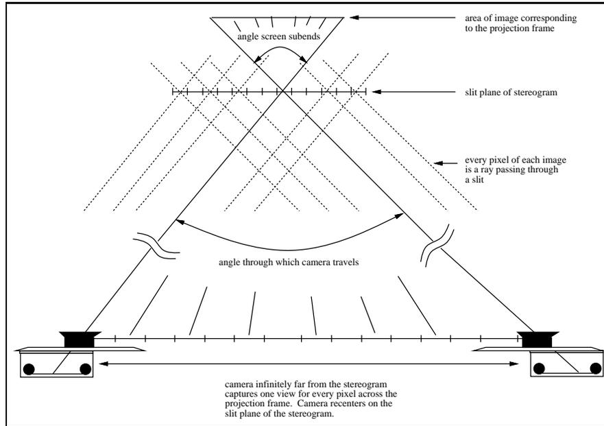
Figure 8: The input camera used to capture perspective views in the infinite camera technique.
