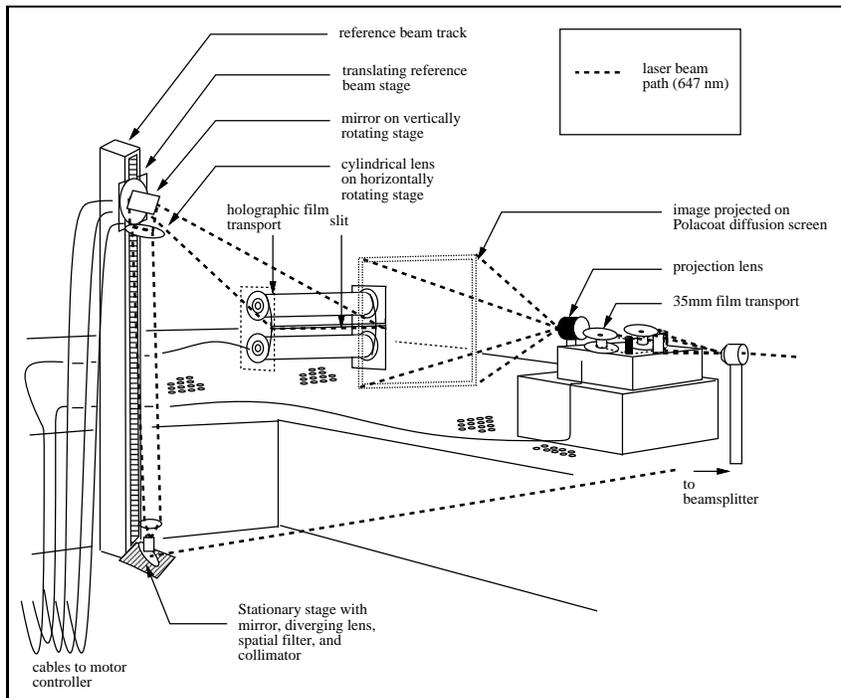
Figure 15: Holographic apparatus used to expose *Large Chevrolet Wheel*.
