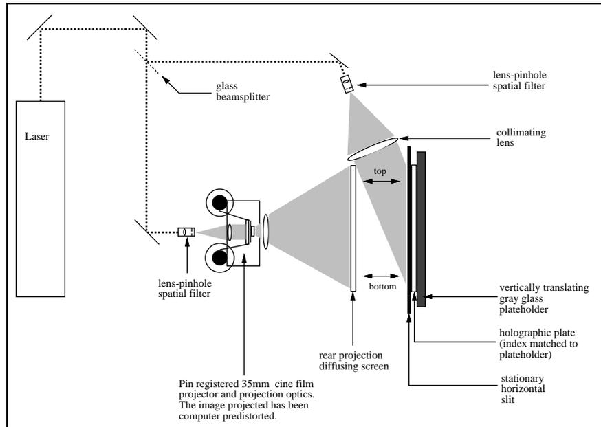
Figure 11: ULTRAGRAM two-step mastering setup.
