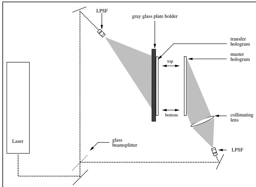
Figure 12: ULTRAGRAM two-step transferring setup, where the transfer is designed for direct illumination.
