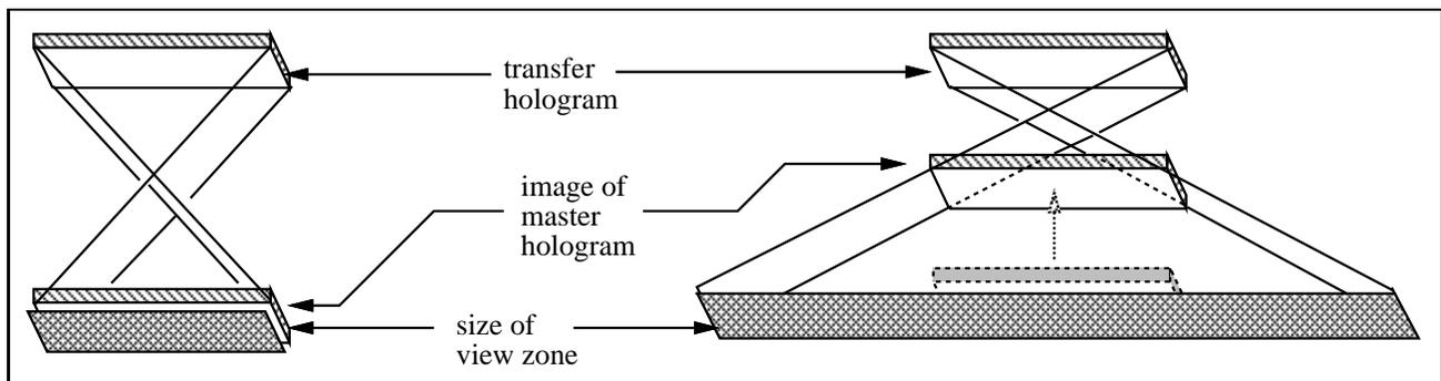
Figure 10: When the plane of the master stereogram is moved away from the viewer and closer to the transfer plane, the size of the view zone widens. Not shown in this picture is the similar widening of the vertical view zone.
