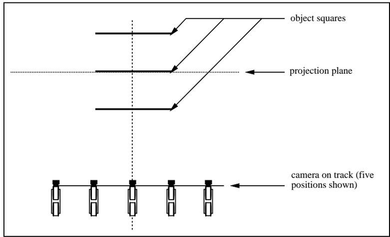
Figure 1: Camera geometry for a simple stereogram.
